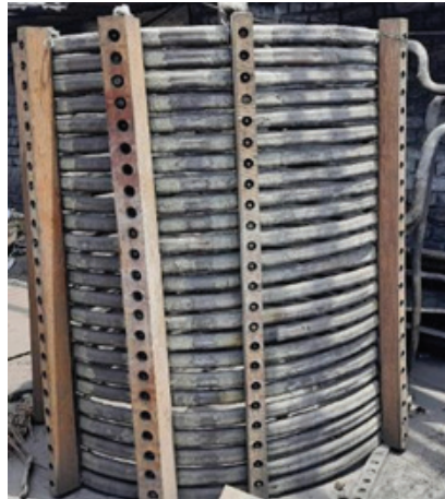
Figure 49 : Pictorial view of copper coil in induction furnace
